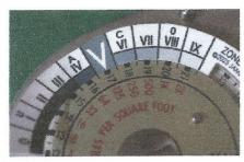
3. On the back of the label, the paper backing has a cut in it so you can remove the backing easily. Remove half of the backing and carefully place the unexposed, non-sticky, half of the label on the meter till the marks of the label match the marks of the meter dial. Remember, Zone V on the label is placed where the red mark is on the dial. (see above) I use the non-sticky half of the label to align the Zone marks. When aligned, I press the sticky side down.
