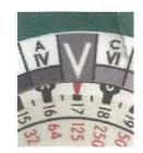
2. On the right side of the label there are some faint gray lines. The lines represent where the Exposure Value (EV) scale window is. If you want to use EVs then you will need to cut out that portion of the label. It is not necessary to use the EV scale to use the Zone System. I will show a label with the EV scale opening for
