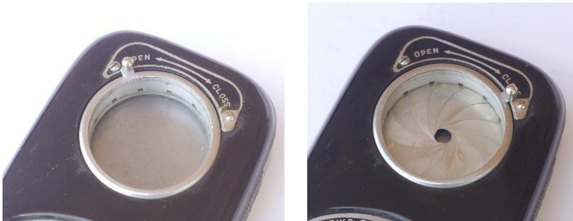
III.1 (left) shows the rear, cell side of the L-V with the aperture lever fully across to the left, the cell completely exposed. III.2 (right) shows the lever across to the right and a small aperture which scales the cell for the higher luminance range on the meter.
