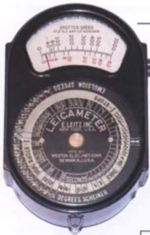
The model 617 Leicameter indicates shutter speeds directly for the default settings. For other settings the inner outward facing pointer is set to the required film speed and the outer inward facing pointer to the indicated shutter speed. Combinations of shutter and aperture values are then read off.
