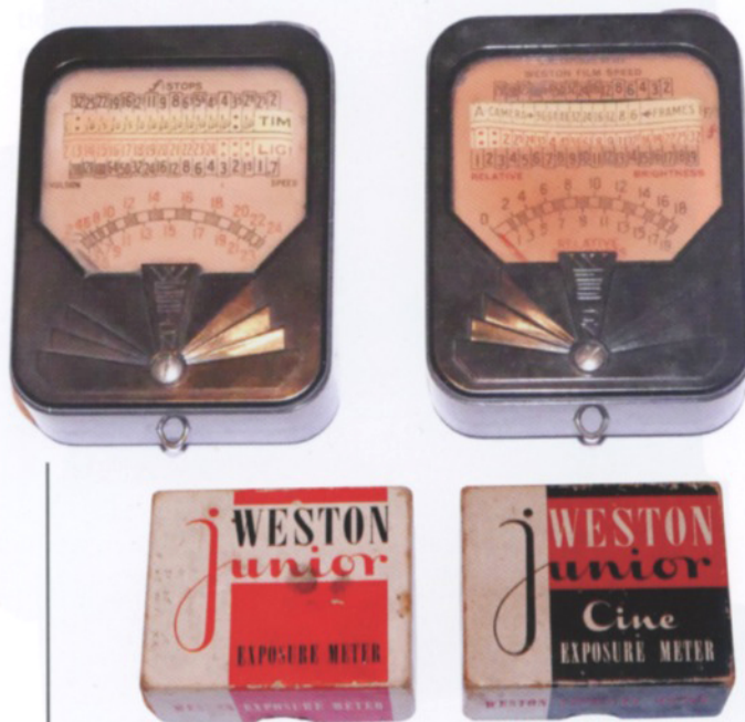
The model 850 Junior and Junior Cine (left to right respectively) at first appear identical. The brightness range mark-up is different and the cine meter uses frames per second in place of shutter speeds.
