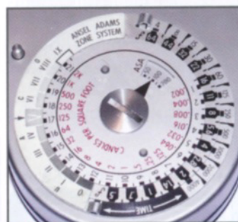
The Ansel Adams variant of the Ranger 9 replaces the E.V. scale on the standard model with a tonal range supporting his Zone System.
