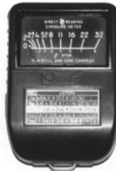
The Model 853 Direct Reading exposure meter of 1954. This is the first model that does not need mechanical readjustment on its front face after each light reading. The meter needle points directly to the aperture required.
