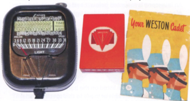
The Model 852 Cadet housed in a more rounded and slimmer casing. In operation the meter is identical to the 850 Junior but the white on black value mark-ups give greater legibility than on the 850. This was the first of any model of Weston meter to use A.S.A. speeds in place of Weston.
