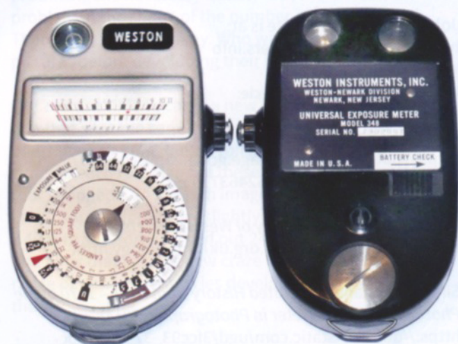
The Cadmium Sulphide based model 348 Ranger 9 sported a larger calculator dial and a spread of 21 luminance capture levels down to 0.002 candles / square foot. A sighting finder is visible at the top. The rear face shows the cell and finder apertures and the battery compartment cover.
