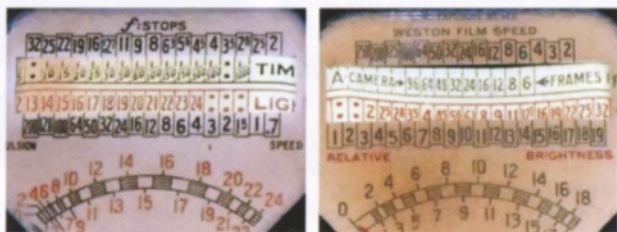
Close up of the 850 Junior meter displays, Universal (left) and Cine (right): The cine meter operation differs from the Universal model in that the luminance scale is marked up in units of Relative Brightness. Frames per second replace shutter speeds, which are aligned to the film stock speed. Lens aperture is then read off against measured light value.
