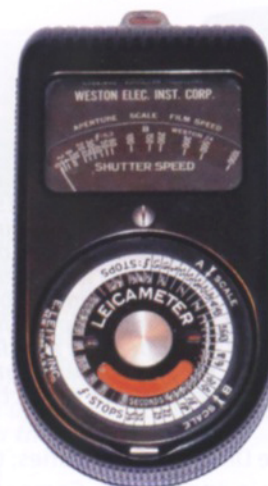
The Model 715 was the last Leicameter made. It now has two pointers for the high and low light level ranges and the Scheiner film speed system has been replaced at last by Weston's own film speeds.
