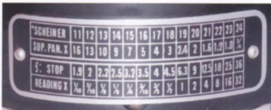
The metal plate round the side of the 627 Leicameter shows two tables. The top table indicates exposure weightings for films of different speeds other than 23 degrees Sch. The lower table gives shutter speed corrections for apertures other than f6.3.
