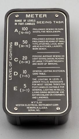
The Westinghouse (Weston) type 801 See-Ability Workplace Light Level Meter. U S Manufacture. c1940
