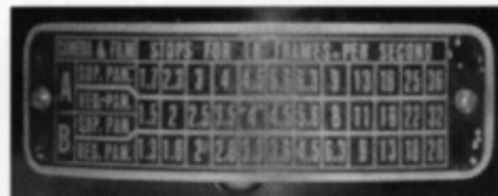
Model 627 Reference Table. Two generic types of panchromatic film are represented here: Regular Pan and the faster Super Pan. The letters A and B refer to the two basic arrangements of the typical rotary shutter. The meter reading is referred to on the centre row and the compensation is read off vertically depending on which combination of film stock and shutter setting is in use.
