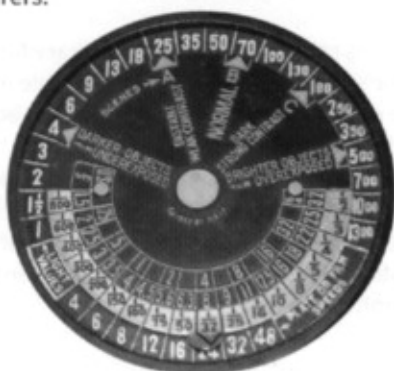
The three-stage calculator dial of the model 617. It has a number of pointers to help the photographer assess their subject. They reference the lightest or darkest subject areas, contrast levels and parameters for over and under exposure.
