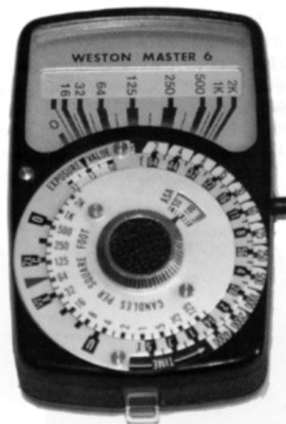
The plastic bodied Master 6 560 from Japan returned to Candles / Square Foot unit markings, had a sliding rather than hinged range baffle, and its own design of invercone.
