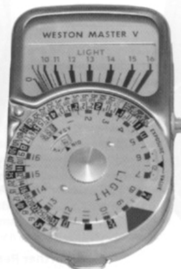
Masters IV, V and the Euro-Master. The Black meter faced model IV 745 (left) dispensed with intermediate exposure markings. They were restored on the long running model V 748 (centre) but dispensed with yet again on the Euro-Master S461.6 (right)
