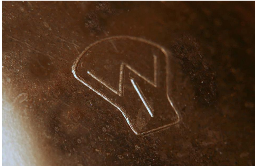
The fan shaped Weston Instrument logo engraved on the inner glass surface of the 856 cell.
