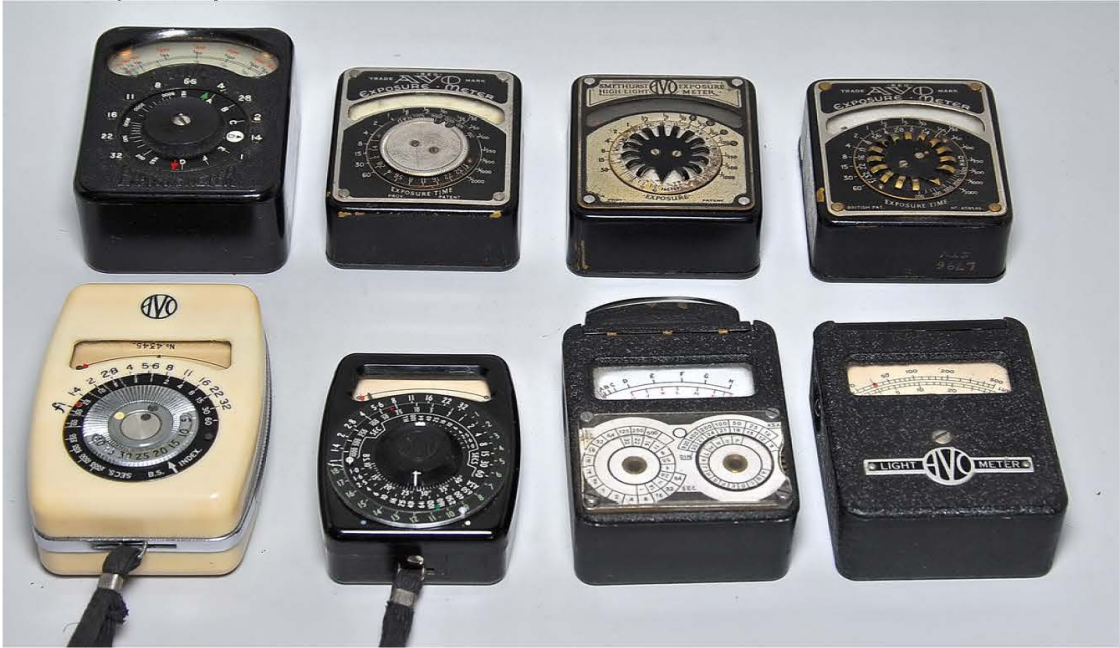
To the left the first AVO meter, the white ring below the selector knob was soon replaced by a black one
