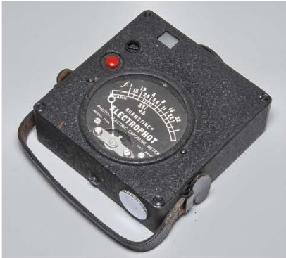
2 nd model Rhamstine Electrophot, with battery, beside without battery. The red button disappeared in the batteryless version.
