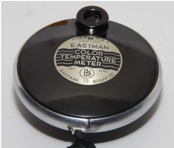
One of the first colour temperature meters was an optical one by Kodak from around 1937.
