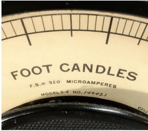
Fig.3 (left): A close up of the Model 24 reveals the range at full-scale-deflection (F.S.) in microamperes (1/1000 th of a milliampere) and a six-figure serial number indicating a late manufacture of the model, probably over more than 30 years. Fig.4 (right): A #5000 cell number is consistent with the production cycle of the Weston model 594 Photronic cell from 1932.
