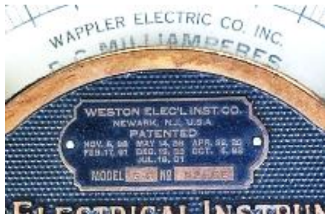
Fig.1(left): The earliest example of the Model 24 Microammeter and the plate listing its patent history, Fig.2 (right). Production date around 1905.
