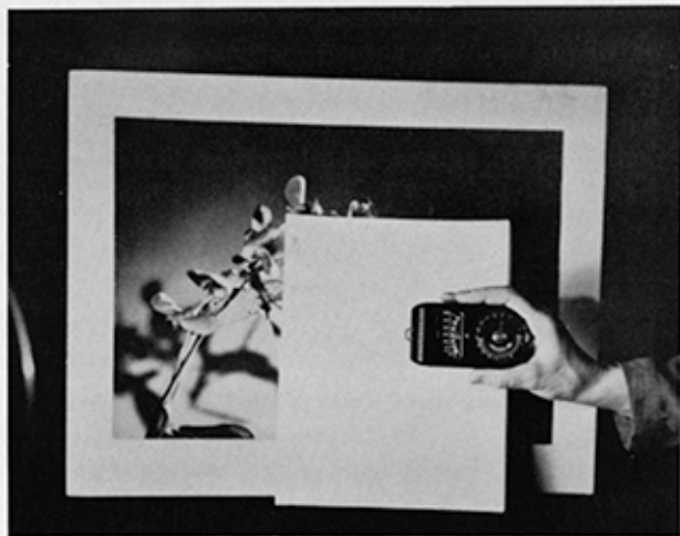
Eliminate the shadow on the white paper by holding the meter at a different angle or changing the illumination
