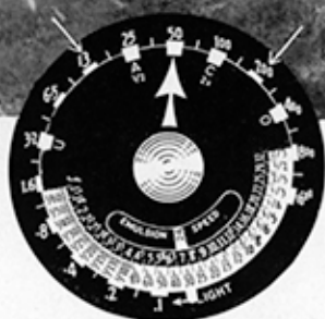
Exposure Guide Dial with normal arrow set midway between the brightness values of 13 and 200.
