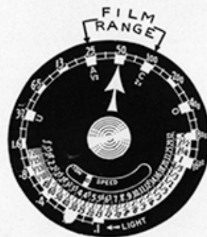
The Exposure Guide Dial showing the color range of the film between positions "A" and "C"
